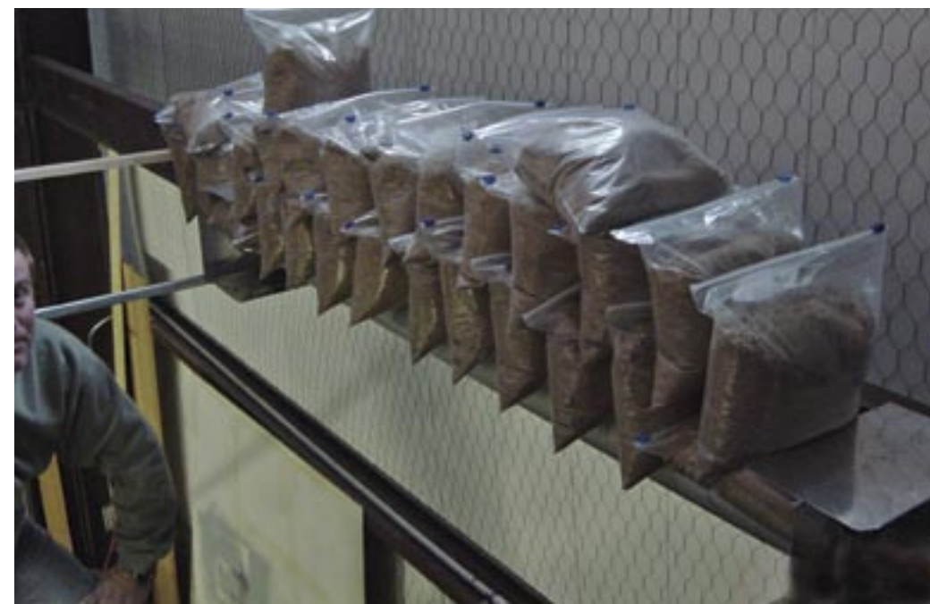
Left: The assembly was tested to 9g without deflection, showing the wing would fail before the tank assembly
