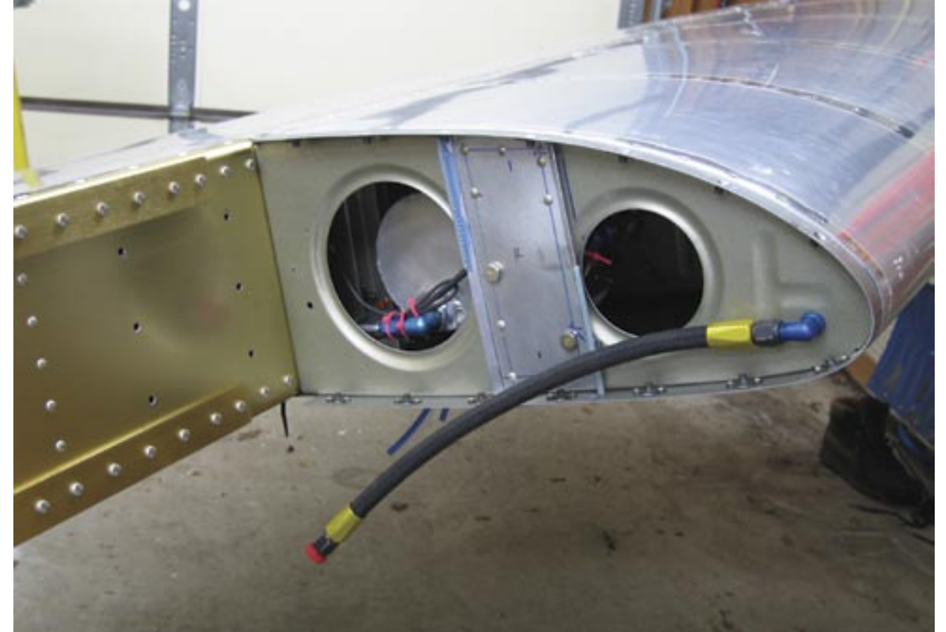
The inboard end of the installed tank, ready to be plumbed into the main tank.
