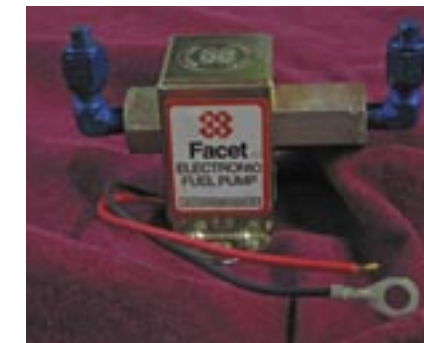
Left: The complete RV-8 kit contains all of the parts needed for installation, including box tanks at the outboard end. The solid-state fuel pump (below) also works as a check valve.
