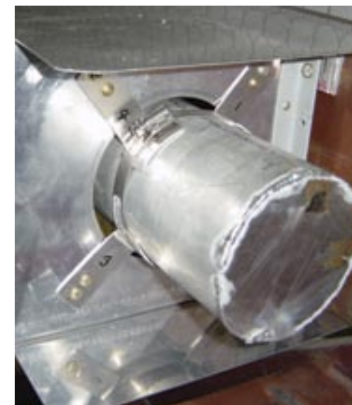
Right: Inboard view of the test mount used to verify the design and installation.
