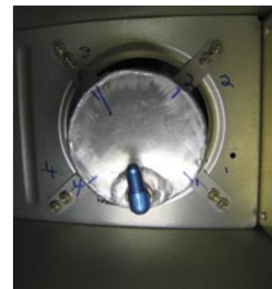
Left: The assembly was tested to 9g without deflection, showing the wing would fail before the tank assembly
